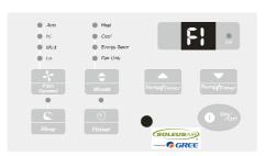
If the display reads "F1" a sensor has failed.
